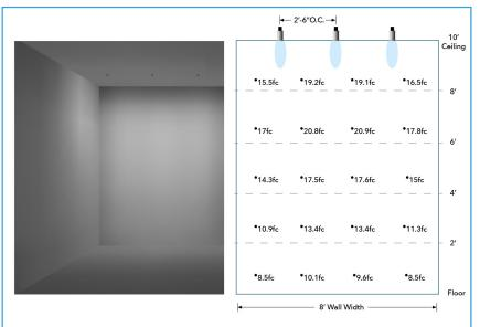
AGI Simulation of 3 Wall Wash fixtures in 8' square room at 10' ceiling height with 2.5' setback and (1:1) 2.5' spacing. Based on Ambient Dim Source at 578 lumens
